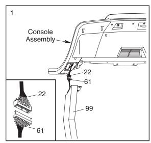
2. Insert the excess Wire Harness (22, 61) down into the right Upright (99).
